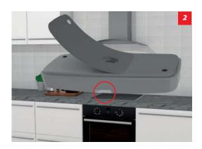
If there is a metal mesh grease filter on the cooker hood, make sure it is free of grease and dry.
